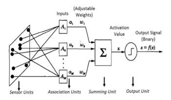
On the basis of sign of the weight of each input, it is decided whether the input has a positive weight or negative weight. The weighted sum of the processing unit produces what we call Activation value and based on the indicator value from activation function, the output is produced.
